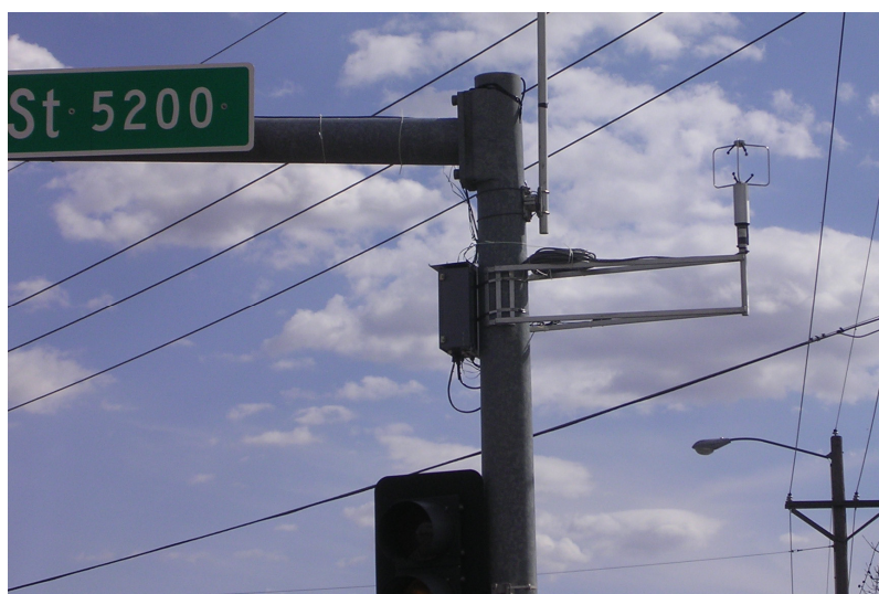
Figure 4.6: Anemometer and data acquisition unit connected to pole
